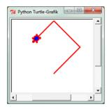
The constructor creates an empty polygon; the polygon maintains a "pen" with color c which is positioned at point (x, y) and is oriented in direction a (angle in radian, 0 is right,  $\pi/2$  is up). By the operation move () the pen is moved distance r into the current direction, adding a line in the pen color to the polygon; by turn(), the pen changes orientation by adding angle a to the current angle; by color() the color of the pen is changed to c.
