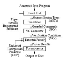
From Leino et al (2002): Extended Static Checking for Java.
