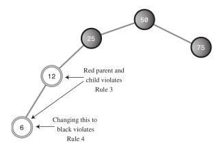
Solution: Rotate right such that 25 is the new root.
