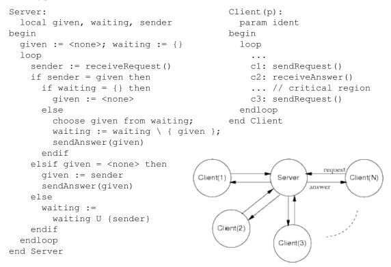
The system operates on the variables given, waiting, sender (describing the internal state of the server component), the variables pc(p) (the "program counter" of client p) and four buffered channels request1, request2, answer1, and answer2 holding the requests sent from each client to the server respectively the answers returned from the server.
